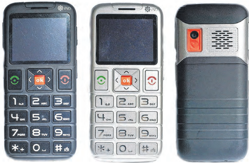
Along with extra-large buttons for easy dialling, the iNO Mobile SOS F12 also has an SOS button which sends out text alerts to up to five pre-programmed mobile numbers when pressed. PHOTO: FORESIGHT TECHNOLOGIES
